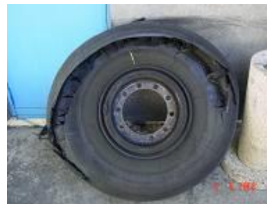
Separation between the casing and the crown
