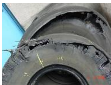
Separation between the casing and the crown
