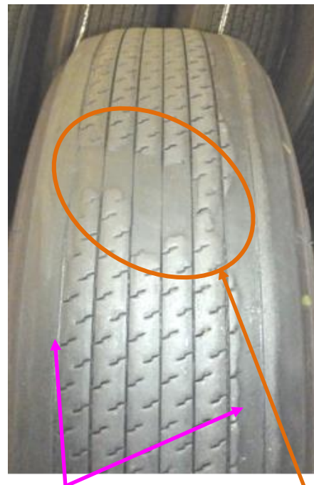
Rail wear and diagonal wear
