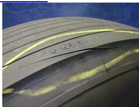
At the shoulder when depth reaches 1 centimeter (0.5 inch)
