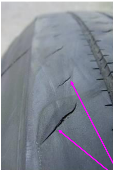
Transversal splits on the tread
